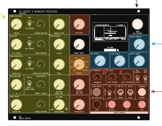
Audio Specs: Stereo audio input and output 32-bit floating point DSP Bit Depth: 8 or 16bit Sample Rates: 8Khz, 11.025Khz, 16Khz, 22.05Khz, 36Khz, 44.1Khz, 48Khz 96Khz Tech Specs: 32HP + 13HP 4.5cm deep 240mA +12V 70mA -12V
