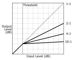
The **ratio** determines how much gain reduction will be applied to the signal once it crosses over the threshold. At a 4:1 ratio, for every 4dB of input signal above the threshold, there will be 1dB of output signal. A 10:1 ratio would output 1dB for every 10dB of input signal, etc.
