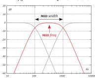
fig. 2: EXAMPLE FREQUENCY RESPONSE
