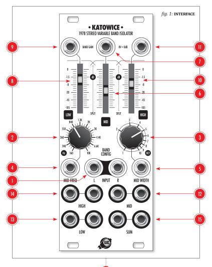
quencies, and the right HIGH slider ① and CV input ① control the high frequencies. The middle band signal is available at the stereo pair of MID outputs ②. Similarly, the low band and high band are available at their stereo pairs of LOW and HIGH outputs ③ and ⑥. A stereo mixdown of the three bands (post-VCA) is available at the SUM pair of outputs ⑥.
