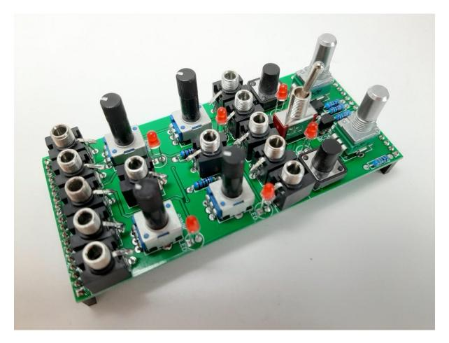
Bolt the metal shaft pots and the sockets to the panel using their nuts and washers. Pop the knobs on the pots and the caps on the sliders. Looks nice huh?
