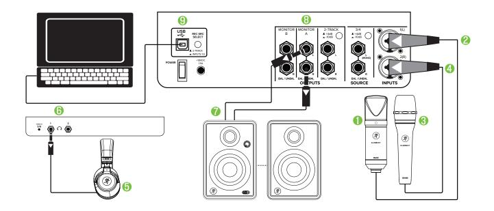
The **EM-91C** condenser microphone ① is connected to channel 1 ② and the **EM-89D** microphone ③ on channel 2 ④ of the **Big Knob Studio**. Check the **Big Knob Studio** manual for tips on getting gains and monitoring set up (This thing has a lot of switches and jacks, the manual is a lifesaver).
