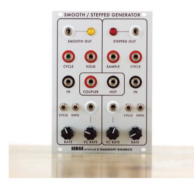
The Smooth section will place a postitve and negative slew on input voltage transitions for lag effects, voltage controlled portamento and for low frequency filter applications." In Cycle-mode (cycle jack patched to the input), the Smooth side "will oscillate yielding a voltage controlled traiangle wave LFO. A high level into the HOLD input will enable the Smooth Function to be used as a trackand-hold circuit with voltage controlled slew rate.
