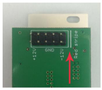
Most modules will come with the cable already connected but it is good to double check the orientation. Be aware that some modules may have headers that serve other purposes so ensure the power cable is connected to the right one.
