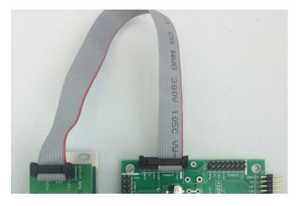
Before reconnecting power and turning on your modular system, double check that the ribbon cable is fully seated on both ends and that all the pins are correctly aligned. If the pins are misaligned in any direction or the ribbon is backwards you can cause damage to your module, power supply, or other modules.
