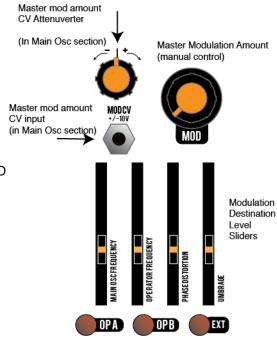
Mixer source selectors (in Modulation Operators section)
