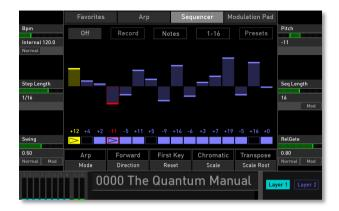
To start the sequencer playback, tap on the **Off** button (it switches to **Running**) and play one or more notes on the keyboard. You can also press the **Arp** button in the Wheel section to start the sequencer.
