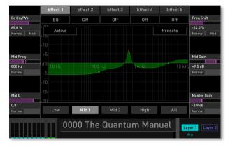
Tap on the corresponding EQ curve in the touchscreen display to edit the **Frequency** and **Gain** parameters. The equalizer features four bands with the following parameters:
