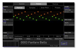
① The Particle parameter page can only be reached, if the Mode is set to 'Granular'. This can be done by tapping on the **Particles** button (and confirming the granular mode switch) or selecting *Granular* with the **Mode** parameter.
