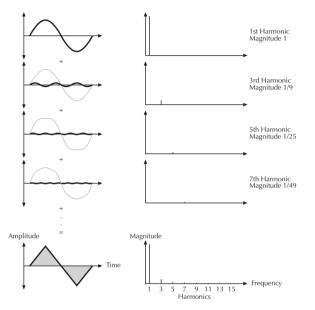
Additive components of the Triangle wave
