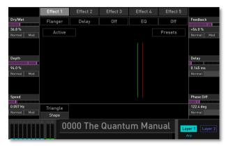
• For the typical Flanger effect sound the **Dry/Wet** parameter should be set to 50%.
