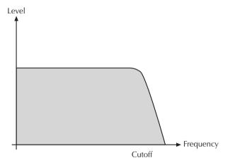
To give you an idea of the extent of damping, consider this example of a lowpass filter: a reduction of 24dB reduces the original level one octave above the cutoff point by approx. 94%. The damping factor two octaves above the cutoff point reduces the original level by more than 99%, which in most cases means this portion of the signal is no longer audible.
