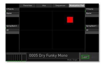
First you need to define the X and Y controller within the **Modulation Matrix**. You can, for example, easily set up a modulation for Cutoff (Pad X) and Resonance (Pad Y).
