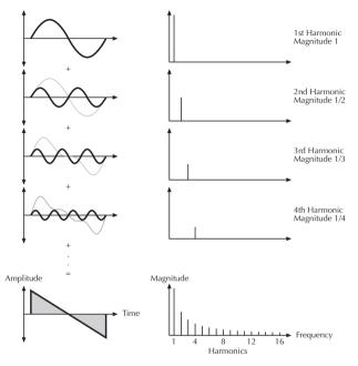
Additive components of the Sawtooth wave
