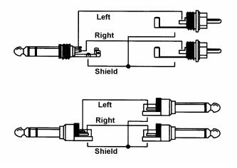
The pin assignment follows international standards. The left channel is connected to the tip, the right channel to the ring of the TRS jack/plug.
