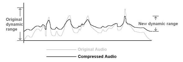
It may be preferred to maintain the quieter passages of audio unaffected and only apply the compression at the highest volume levels, set by a "Threshold" parameter. This is known as "Limiting" and can be useful to control maximum sound levels for safety of listeners and to protect audio equipment.
