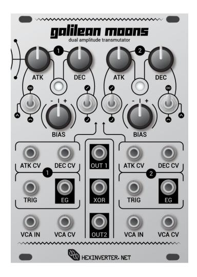
**ATK CV:** This input responds to 0-5V CV and alters the duration of the attack/upwards slope of the envelope. Higher CV = longer duration, lower CV = shorter duration. The response of this input is NOT perfectly linear as this allows for a more useful range of envelope times to be used. **This input expects slowly moving CV signals and may respond in a chaotic manner if driven at higher (ie: audio) frequencies, but feel free to experiment!**
