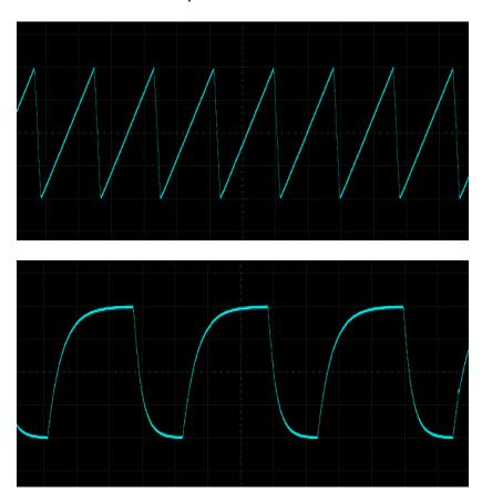
Dynamic LFO waveforms can be generated by varying the SHAPE control and applying voltage control to the ATK/DEC inputs over time:
