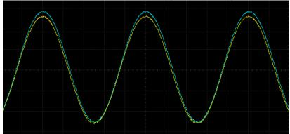
The output waveform is adjusted too low:
