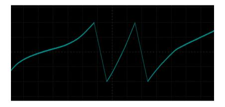
The LFO can be synced to a clock signal by resetting the LFO with the clock signal at the TRIG input. This is a freely running linear LFO:
