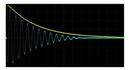
You can also modulate signals (blue) in a linear fashion as well, via linear CV (yellow):
