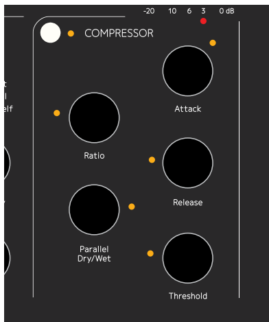
Compressor section on the Console 1 hardware.
