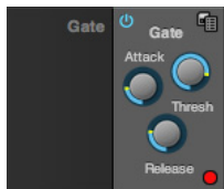
Figure 8-2: The Gate module.
