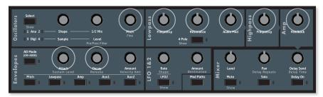
The eight parameters are Oscillator Pitch, Lowpass Frequency, Lowpass Resonance, Audio Mod, Highpass Frequency, VCA Feedback, Envelope Attack and Envelope Decay. For each of these eight parameters, moving the knob causes the playback of all sounds to be altered simultaneously. Because the parameter values can be very different for different sounds, the individual parameters are moved proportionally in a way that results in the overall change sounding very natural.
